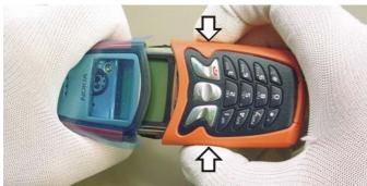
To open the unit the A-Shell has to be removed first. Press the grip markings on both sides of the B-Shell and pull the A-Shell apart from the B-Shell.
