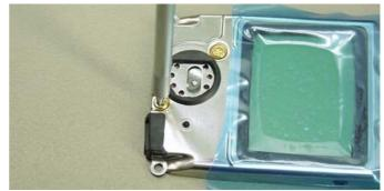
It is also possible to change the speaker, if needed. Therefore you have to unscrew these two screws. Remember to use torque of 8 Ncm when tightening the speaker screws.
