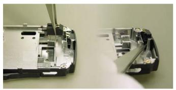
The Vibra Motor with its rubber case is squeezed into the B-Cover like the Microphone. Do not grab the spring connectors, because they may be damaged when pulling the microphone. To change the Microphone, push it up carefully with tweezers.
