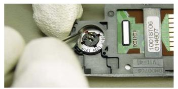
Replace the protection foil. Now you have the separated plastic frame of the LCD unit. You can now carefully push out the speaker with your fingers or tweezers.
