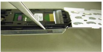
Remove the protection foil of the display and unlock the snaps on both sides of the display frame.
