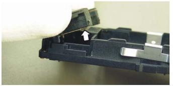
Move up the antenna as shown in the picture. Take care not to damage the antenna contacts. The metal is very sensitive against corrosion, so please don't touch the metal with your fingers. Use gloves instead.
