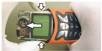
Now, press the release springs near the display and pull the unit out of the B-Shell.
