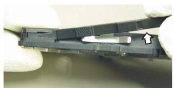
Pull up the lower side of the Release Spring and take it out of the upper holder.
