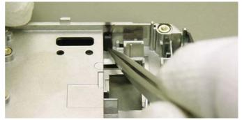
For changing the plastic Release Springs the lower sides have to be unlocked first.
