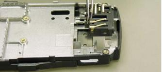
When the SIM Connector is removed, the DC + HF Connector can be taken away.
