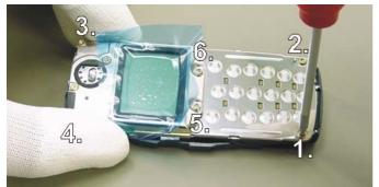
Remove the six screws with screwdriver Torx T6 in the shown order. When assembling the reverse order has to be taken with torque of 17Ncm.
