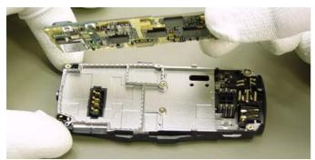
All the connectors are located under the CMT module. Take care that the RF Gasket stays in position on the four guiding pins. If the gasket is bent it has to be changed.
