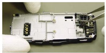
The SIM Connector can be removed with tweezers.
