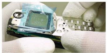
Now the LCD module can be removed easily.
