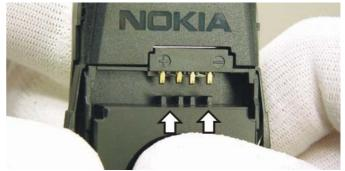
With the Battery Connector Extractor Tool SRT-3 used in 8210 you can easily push out the Battery Connector without bending the sensible contacts.
