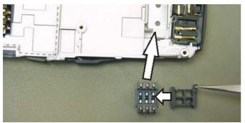
If you assemble the SIM Connector, be aware that the Twin Rip is also fitted correctly. The Twin Rip is responsible to keep the SIM Connector in the right position.
